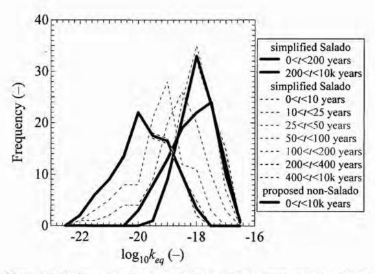
Figure 4: Thick lines show the proposed distributions for the simplified shaft model. The simplified model would include only one material property change at 200 years for the Salado component of the seal. The permeability distribution proposed for non-Salado material is simply the equivalent permeabilities from the baseline shaft seal model.
